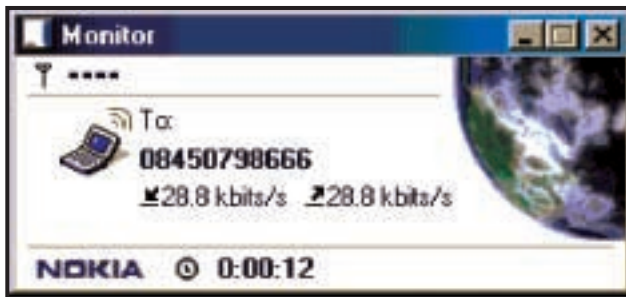
HSCSD technology enables the Nokia 6210 to transmit and receive data at higher speeds than older mobile phones
